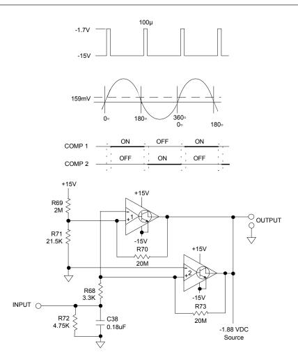
Figure 5-1. Two-Comparator OR Circuit
